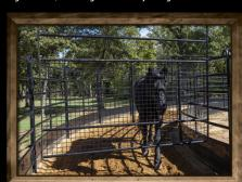
**DIVIDER PANELS-** Low impedance electrically-charged. free swinging divider panels encourage horses that have a tendency to lag behind to keep pace. Each divider panel is made of heavy duty 2"x2" 4 gauge wire mesh, and the electrical charge is optionally activated at the control box.
