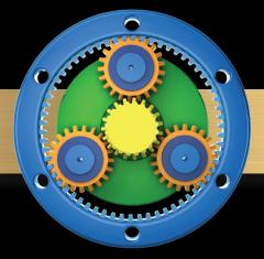
**PLANETARY GEAR BOX** - Never worry about burning belts again. Priefert Walkers run on a planetary gear box system similar to those used in heavy earth moving equipment like track hoes. This provides years of virtually maintenance free, reliable operation.
